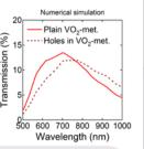
Our code solves the Maxwell equations as an eigenvalue problem via plane-wave decomposition, and propagates the solution across the different layers by means of *transfer matrices*, which contain the continuity conditions for electromagnetic field components at an interface. Hole arrays are represented by the Fourier transform of the piecewise dielectric permittivity.
