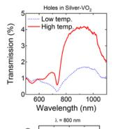
The zero-order transmission (i.e., detected beam collinear with incident beam) of hole arrays in  $Ag\text{-VO}_2$  (left) and  $Au\text{-VO}_2$  (right) exhibits typical EOT profiles. Through the  $VO_2$  phase transition, the EOT intensity can be switched "on/off" in the near-IR.
