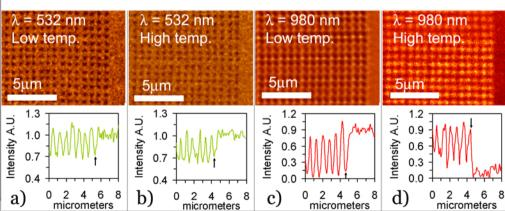
NSOM images of far-field transmission through a  $VO_2$  hole array, under near-field illumination, and corresponding plots of intensity vs. position along a section of a row of holes and extending into the plain-film area; the rightmost hole is indicated by an arrow in each plot. Only in the metallic phase and under near-IR light do the apertures appear brighter (i.e., transmit more) than the plain film.
