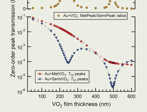
FEM | Hole Arrays in Gold+VO<sub>2</sub> on Glass: *Thickness VO*<sub>2</sub>
